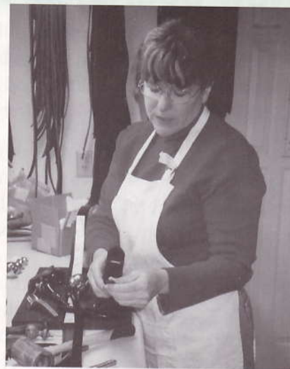
DeeAnna Weed demonstrates how she laces a narrow bell strap through a wider liner strap before attaching the restored vintage bells. Straps made at Classic Bells are constructed of high quality bridle leather and can actually be used on horses or for decorative purposes.
