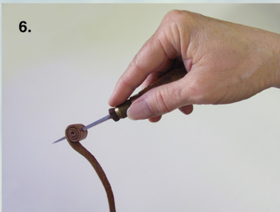
When roll is approaching tail, stop. Then take large diamond bladed awl and stab a horizontal slit through entire roll.
